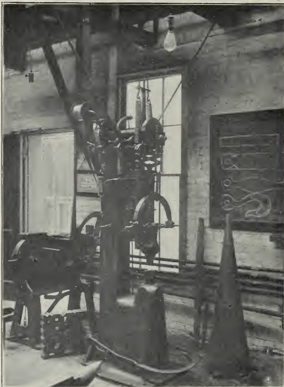
A Corner in the Blacksmith Shop, Showing Power Shears and Power Hammer.
